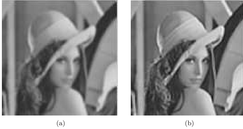
FIGURE 5.1. Image (a) shows a blurred image of Lenna blurred using a Gaussian kernel with \sigma = 1 . Image (b) shows the result of the deblurring IDE model (5.4), as t \rightarrow \infty .
