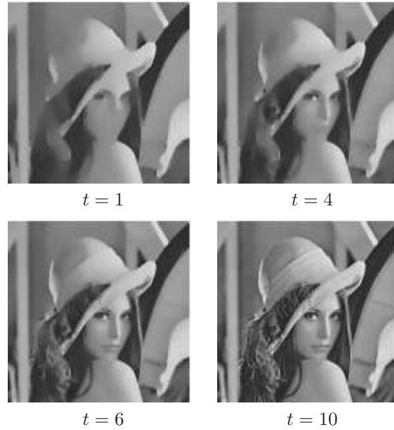
FIGURE 4.1. The images, U(t) = \int_0^t u(\cdot, s) ds , for the modified IDE (4.1) at t = 1, 4, 6, 10 . Here \lambda(t) = 0.002 \times 2^t .
