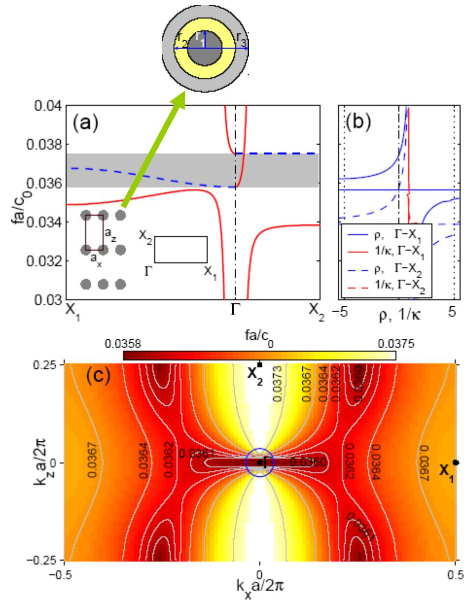
By arranging isotropic resonators in an anisotropic lattice (e.g. rectangle), we can get anisotropic response.
