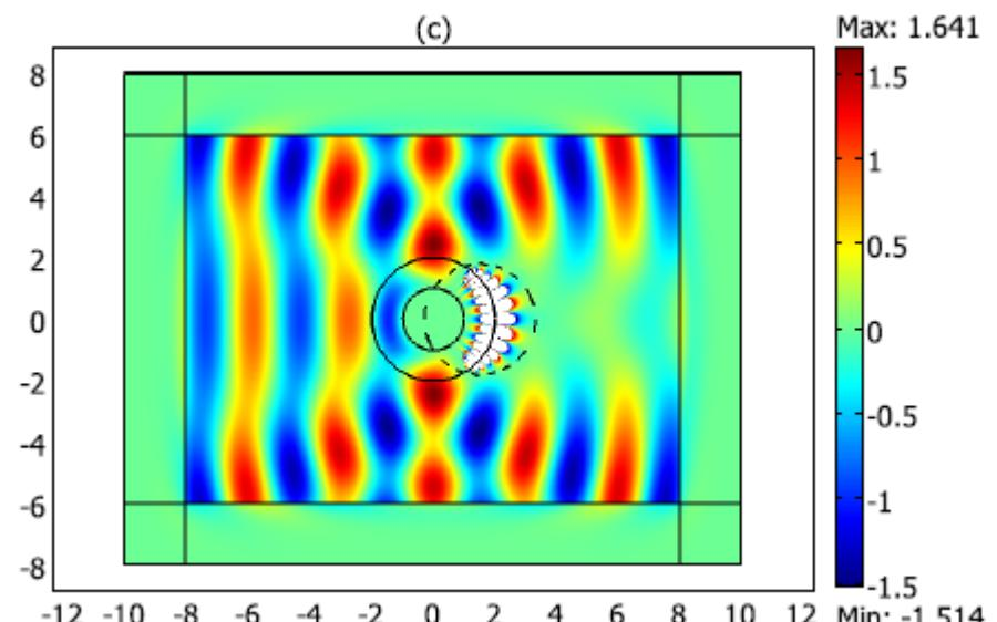
A cylinder with a different radius at origin, coated with the transformation media shell
