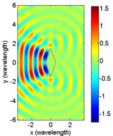
Cloak reduces the cross section of the diamond-shaped domain to that of a thin-plate
