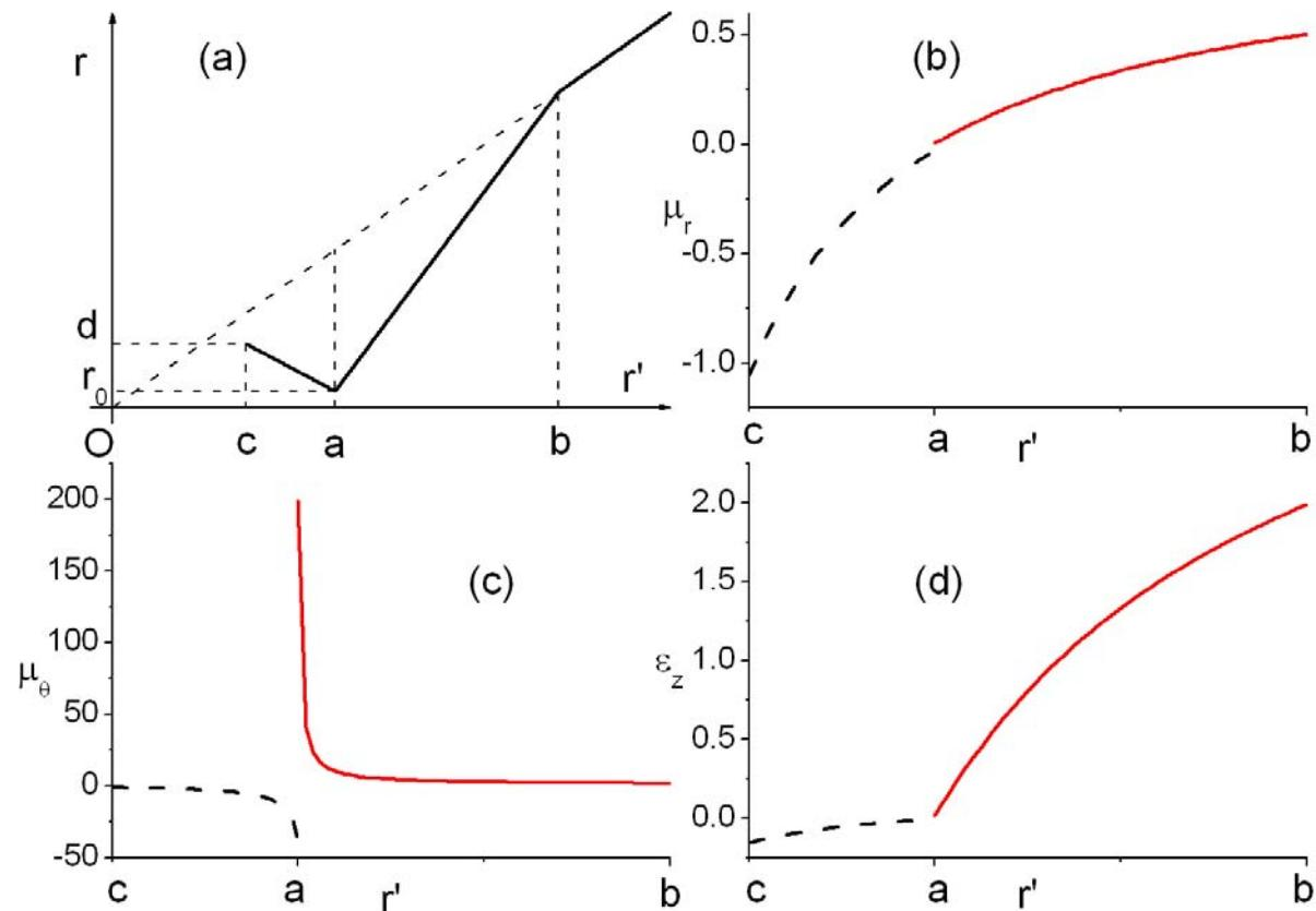
(a) The coordinate transformation of the cloak and anti-cloak: [a,b] is the cloak [c,a] is the “anti-cloak”. They are in direct contact. Note that “anti-cloak region has negative parameters
