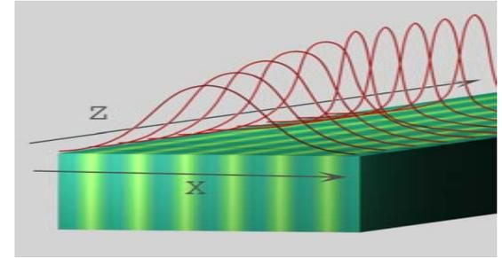
$$iA_z(z, \vec{x}) + \nabla^2 A + (1 - V_{nl}(\vec{x})) F(|A|^2) A - V_l(\vec{x}) A = 0$$
