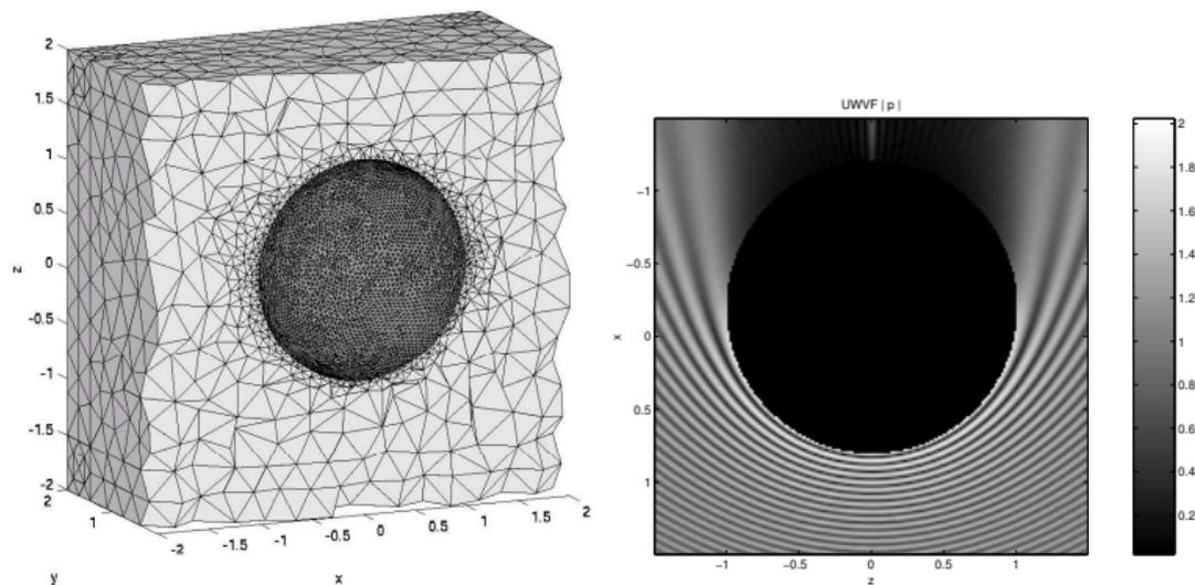
*Left:* The mesh. *Right:* The UWVF approximation for a plane wave at  $\kappa a \approx 63$ .
