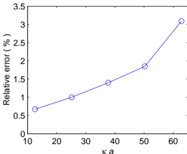
The results are computed in the same mesh using the condition number limit  $\text{Max}(\text{Cond}(D_k)) < 1e6$ . Note, the total error includes errors due to UWVF approximation, PML and triangulated surface of the sphere.
