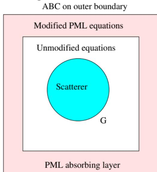
The PML layer absorbs incident waves exponentially rapidly. The only reflection is from the outer boundary (for the continuous problem).
