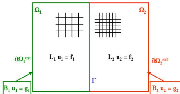
$$\left\{ \begin{array}{ll} L_1 u_1 = f_1 & \Omega_1 \times [0, T] \\ u_1 \text{ given} & \text{at } t = 0 \\ B_1 u_1 = g_1 & \partial\Omega_1^{\text{ext}} \times [0, T] \\ C_1 u_1 = C_1 u_2 & \Gamma \times [0, T] \end{array} \right. \quad \left\{ \begin{array}{ll} L_2 u_2 = f_2 & \Omega_2 \times [0, T] \\ u_2 \text{ given} & \text{at } t = 0 \\ B_2 u_2 = g_2 & \partial\Omega_2^{\text{ext}} \times [0, T] \\ C_2 u_2 = C_2 u_1 & \Gamma \times [0, T] \end{array} \right.$$
