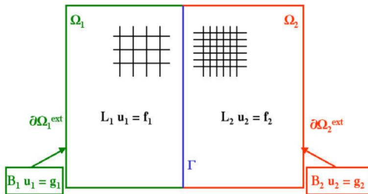
$$\begin{cases} L_1 u_1^{n+1} = f_1 & \Omega_1 \times [0, T] \\ u_1^{n+1} \text{ given} & \text{at } t = 0 \\ B_1 u_1^{n+1} = g_1 & \partial\Omega_1^{\text{ext}} \times [0, T] \\ C_1 u_1^{n+1} = C_1 u_2^n & \Gamma \times [0, T] \end{cases}
