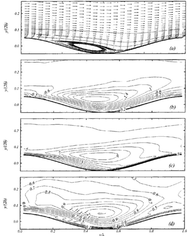
Figure 12. Wavy channel,  $2a/\lambda_s = 0.1$ ; CIW simulation. (a) Mean velocity vectors and streamlines; (b) Reynolds stress  $\langle u'v' \rangle$ ; (c)  $q^2$ ; (d) normalized eddy viscosity.
