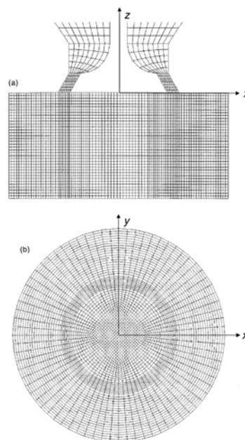
Fig. 2. Two-dimensional sections through computational mesh for the axisymmetric piston-cylinder assembly of Morse et al. [27], including coordinate system definition. (a) Cross section through the axis of symmetry ( $y = 0$ ). (b) Cross section normal to the axis of symmetry ( $x = \text{constant}$ ).
