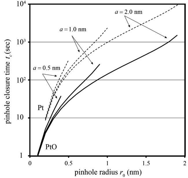
Fig. 3 Pinhole closure time  $t_c$  vs initial pinhole radius  $r_0$  for different values of the pinhole edge radius of curvature  $a$ . PtO-terminated surfaces: thick lines; Pt-terminated surfaces: thin dashed lines.
