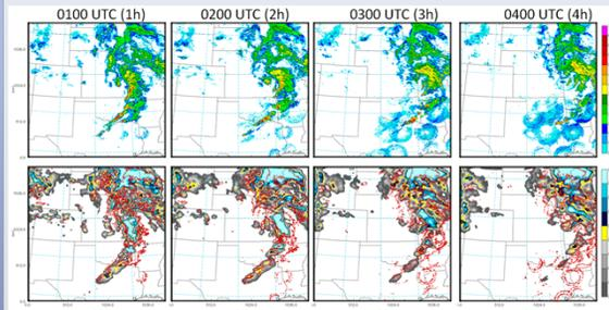
Figure 4. Observed reflectivity (top) and neighborhood (radius = 10 km) ensemble probability of forecast reflectivity exceeding 15 dBZ (bottom) at model grid level 20 at (left to right) 0100, 0200, 0300, and 0400 UTC, corresponding to 1-, 2-, 3-, and 4-hour forecast, valid at 0100, 0200, 0300, and 0400 UTC, 11 May 2010, respectively. The 15 dBZ radar reflectivity contour observed by the WSR-88Ds at the same time is in red contour.
