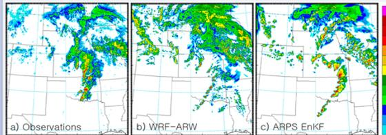
Figure 3. (a) The observed radar reflectivity mosaic; (b) CAPS real-time WRF-ARW forecast; and (c) deterministic forecast from the EnKF ensemble mean analysis at model grid level 20 (about 3.6 km above mean sea level) for the central US domain, corresponding to 5-hour forecasts, valid at 2300 UTC, 10 May 2010.
