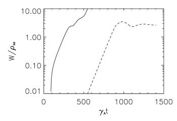
FIG. 6. Island widths  $w/\rho_{se}$  vs  $\gamma_A t$  for  $T_i/T_e$ =5 with (solid) and without (dashed) added initial noise in the simulation. The nonlinear saturation is avoided for very weak levels of initial noise.
