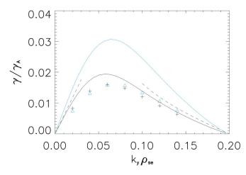
FIG. 1. (Color online) Linear growth rates  $\gamma/\gamma_A$  vs  $k_y\rho_{se}$  for case I with  $\gamma_A$  given by Eq. (10) and  $\rho_{se}=c_{se}/\Omega_{ci}$ . The "+" are GS2 values for  $T_i/T_e \ll 1$ , triangles  $T_i/T_e = 5$ . The left and right dashed lines are Eqs. (10) and (11), respectively, with  $T_i = 0$ . The solid lines are the numerical solution of a reduced four-field fluid model for  $T_i = 0$  (lower) and  $T_i = 5T_e$  (upper).
