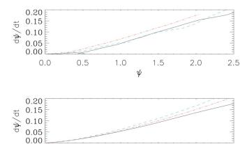
FIG. 5. (Color online) Gyrokinetic (upper panel) and two-fluid (lower panel) nonlinear reconnection rates for case II vs  $\psi$ , the reconnected flux inside the island, for  $T_i \ll T_e$  (solid line),  $T_i = T_e$  (dotted-dashed),  $T_i = 5T_e$  (dashed)
